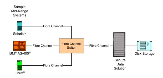
The Secure Data Solution is a totally outboard system that replaces tape drives and does not require the installation of agents on the midrange server. Because there are no agents on the server, the solution integrates seamlessly with most of the midrange backup software in use today, including Tivoli Storage Manager, Net Backup, Veritas, etc. Likewise, it has the flexibility to replace locally attached tape drives including Fibre Channel/SCSI-attached 3590- and LTO- series tape drives.
